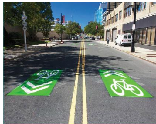
Shared-lane markings typically consist of a bicycle and chevron symbol (photo above left). To increase the visibility and effectiveness of the marking, the marking can be applied on a green background, such as the example from Newark shown above. This “enhanced” shared-lane marking is particularly useful on streets with higher traffic volumes and more activity. Additional design details can be found in NACTO’s “Urban Bikeway Design Guide.”
